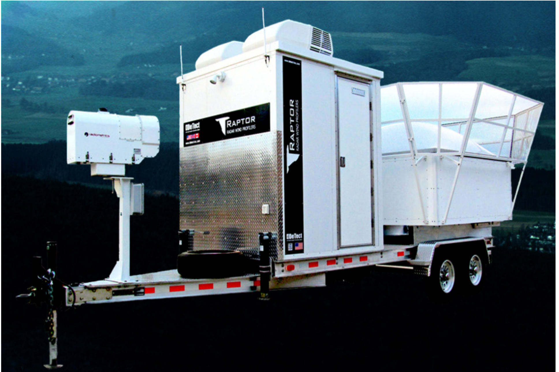
San Diego Gas & Electric operates two mobile wind and thermodynamic profilers for Santa Ana wind, fire weather, solar and utility load forecasting ( Newscast )
