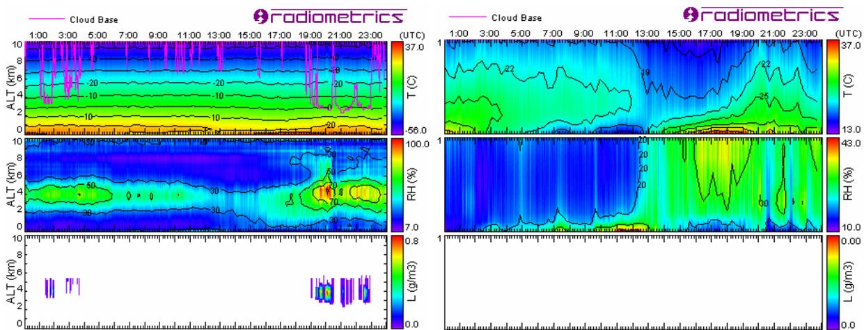
Figure 2. Radiometric temperature, humidity and cloud liquid profiles to 10 km (left) and 1 km (right) height 11Jun07 (UT) at Denver. Cloud base height is indicated by the magenta line.
