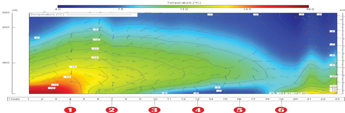
Figure 5. Diurnal evolution of boundary layer temperature and wind at North Las Vegas Airport displayed real-time by RDX-RAOB software.
