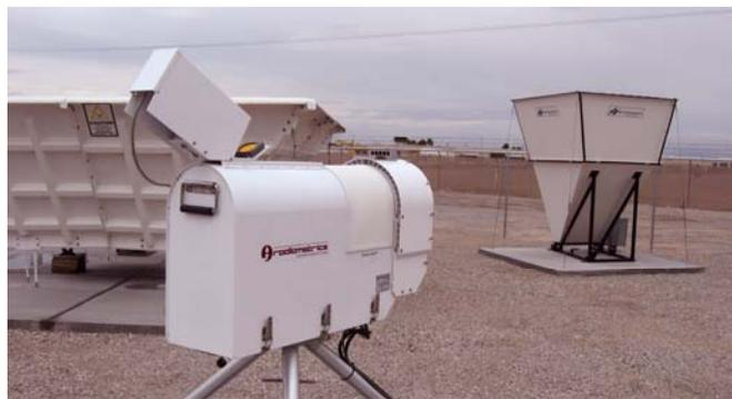
Figure 3. Wind radar, radiometer and sodar (left to right) operated by the Clark County Department of Air Quality and Environmental Management.
