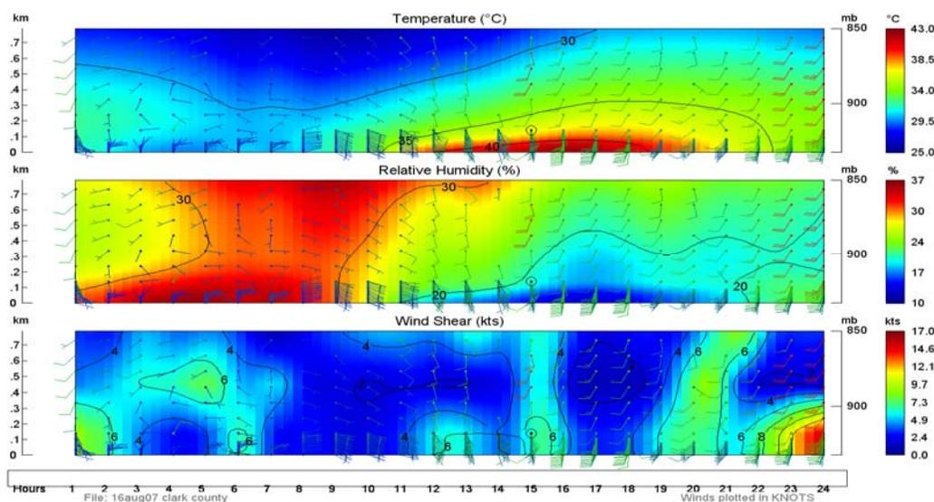
Figure 4. Boundary layer temperature, relative humidity and wind shear at North Las Vegas Airport automatically displayed real-time by RDX-RAOB software.
