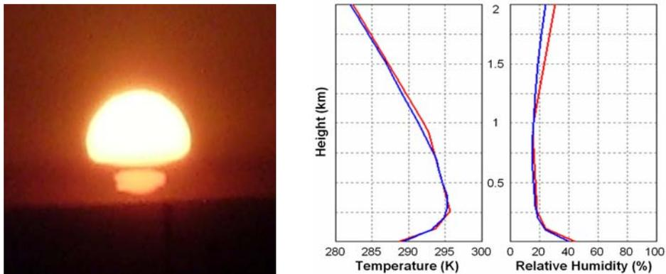
Figure 1. Sunrise (left) with radiometer (blue) and radiosonde (red) temperature and humidity profiles (right), at 6 am local time 11 June 2007, Denver, Colorado.
