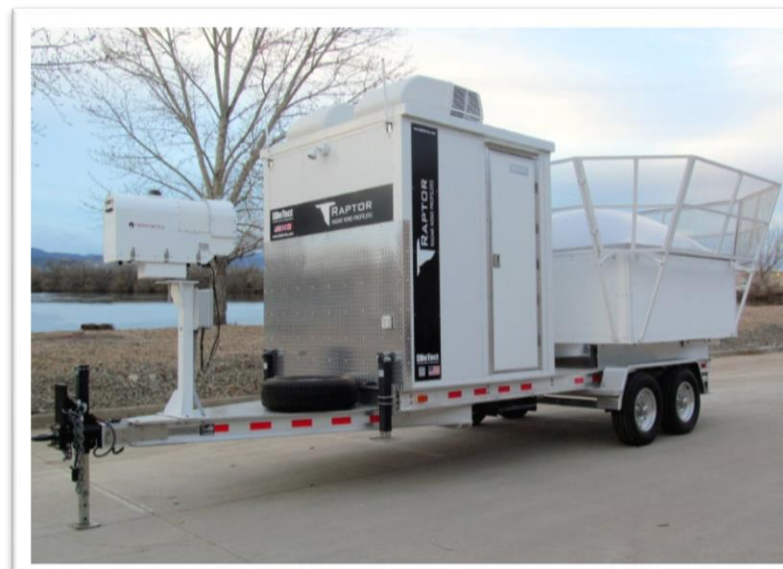
RAPTOR XBS-BL Portable Boundary Layer RWP with optional Radiometer.
