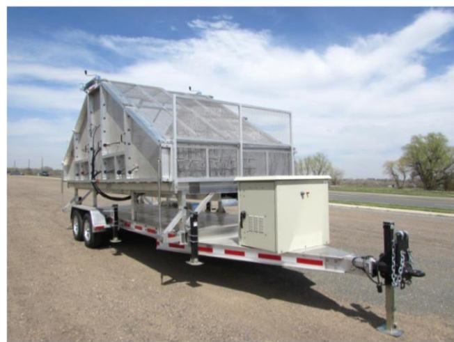
RAPTOR FBS-T 449 MHz 73e-2kW Tropospheric RWP antenna folded for transport (left) and set up for transmission (right).
