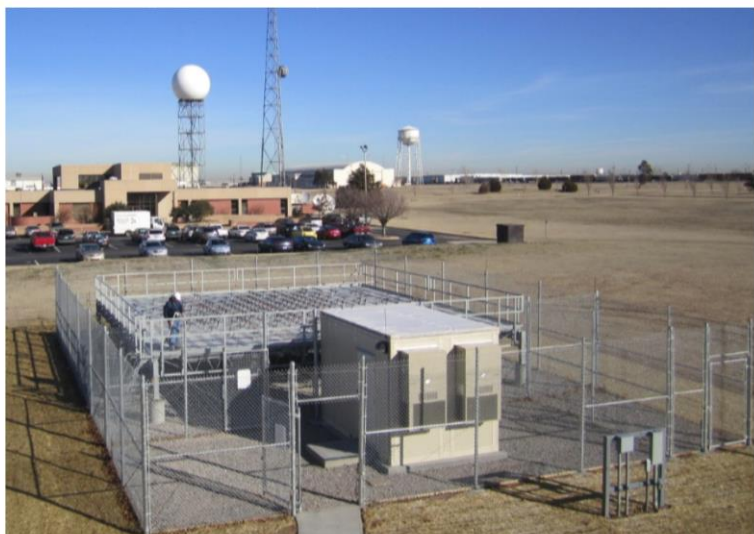
RAPTOR FBS-ST 256e-12kW Stratosphere-Troposphere Radar Wind Profiler designed and built for the US National Weather Service.
