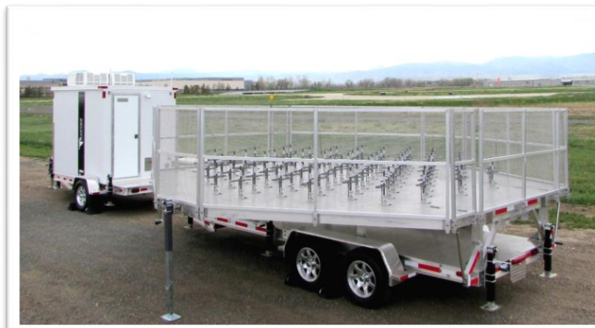
RAPTOR FBS-T 449 MHz 73e-2kW Tropospheric RWP antenna folded for transport (left) and set up for transmission (right).
