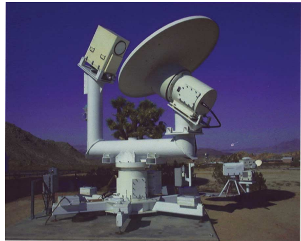
Fig. 6. A photo of the Cassini Media Calibration Subsystem taken at DSS-13 in Goldstone, CA. The new advanced WVR is seen in the center and the MTP and J-series WVR are shown in the background to the right. The WVR antenna is a 1-m-diameter offset parabolic reflector with a 1° beamwidth.
