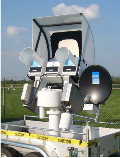
Fig. 1. ADMIRARI radiometer. On the right side, (black antenna) a micro-rain radar system is installed.
