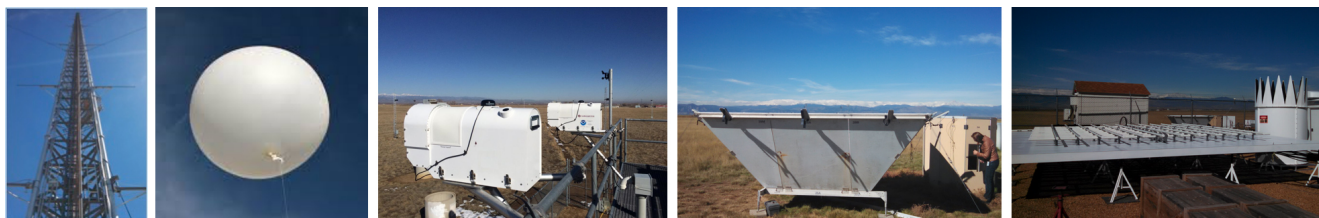
Figure 1. Instruments used in this study. From the left: 300 m equipped meteorological tower (photo credit: Katie McCaffrey), radiosonde, 2 MWRs, 915 MHz and RASS system (photo credit: Katie McCaffrey), 449 MHz and RASS system (photo credit: Katie McCaffrey).
