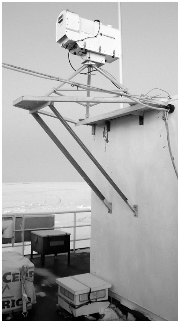
FIG. 1. The MWRP mounted on board the CCGS Amundsen .
