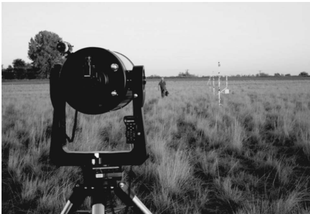
Fig. 2. Experimental setup with the 14-in. telescope, ultrasonic anemometer, and self-logging thermometers at BAO.
