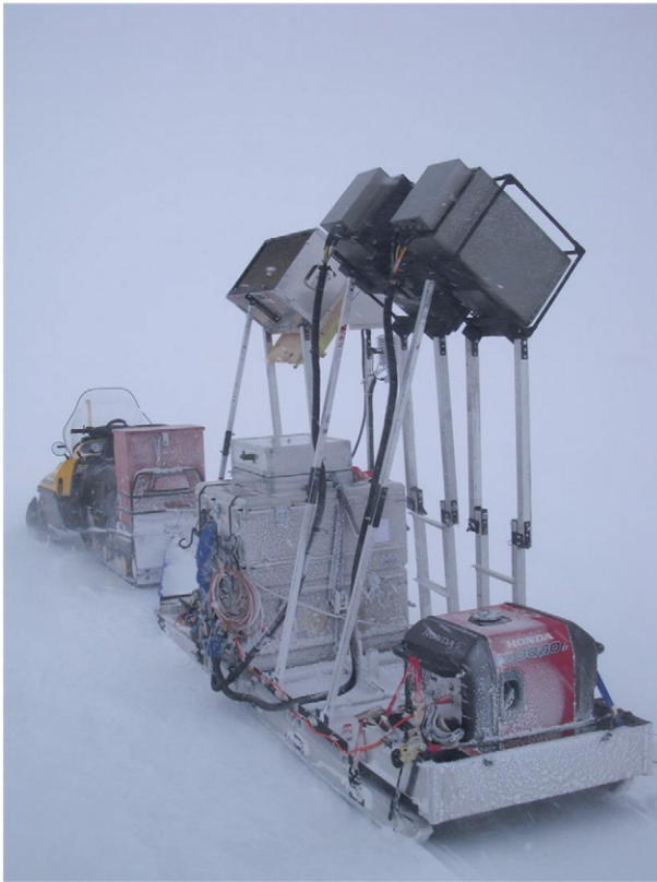
Fig. 2. The Environment Canada sled-based microwave radiometer system in measurement configuration.
