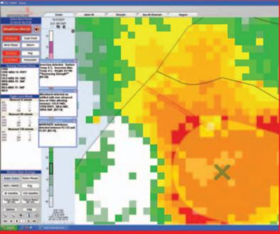
The AWDSS takes all available data and uses a set of complex algorithms and forecasting techniques to produce 'nowcasting' products, presented on a single situation display.
