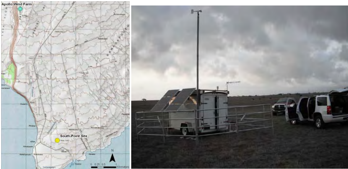
Figure 4.4 Solar powered, mobile SODAR with met-mast at South Point.
