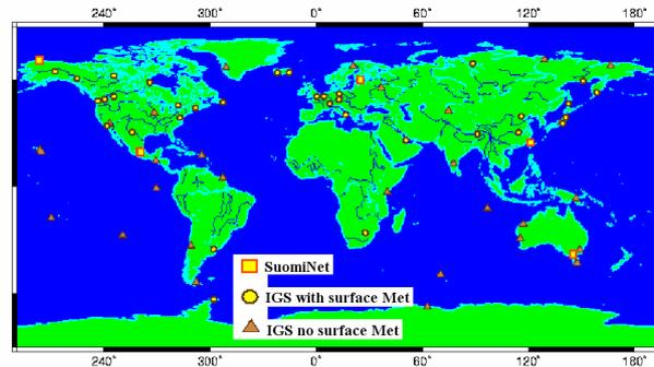
Figure 12. Global GPS networks providing atmospheric sensing<sup>29</sup>. Only IGS<sup>30</sup> sites are shown in the continental U.S. and Canada.
