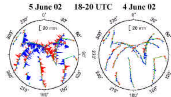
Figure 5. Unmodeled GPS residual slant delays at Lamont Oklahoma during stormy and stable conditions. Zenith is plot center and the horizon is the perimeter. Residuals are plotted about the satellite ground track axis (green). Red represents excess slant delay with respect to modeled slant delay, and blue is less.
