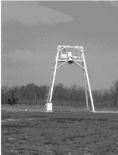
Fig. 1. LEWIS on its supporting structure and with rotating mechanism. The rotation axis is 13.6 m high. The length of LEWIS is 3 m, and the weight is about 200 kg.
