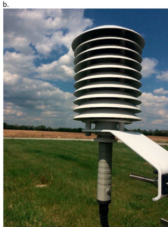
FIG. 4. (a) Aspirated radiation shield (Mahmood and Foster 2008) and (b) Gill radiation shield (naturally ventilated).
