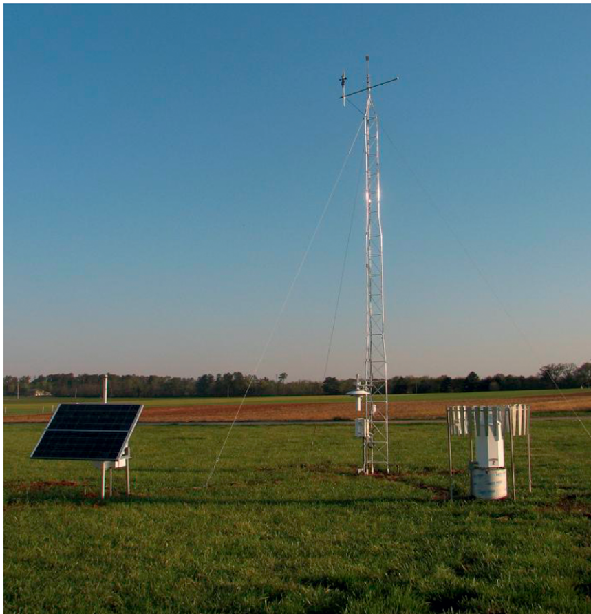
FIG. 3. A mesonet station in Kentucky with good exposure (Mahmood and Foster 2008).
