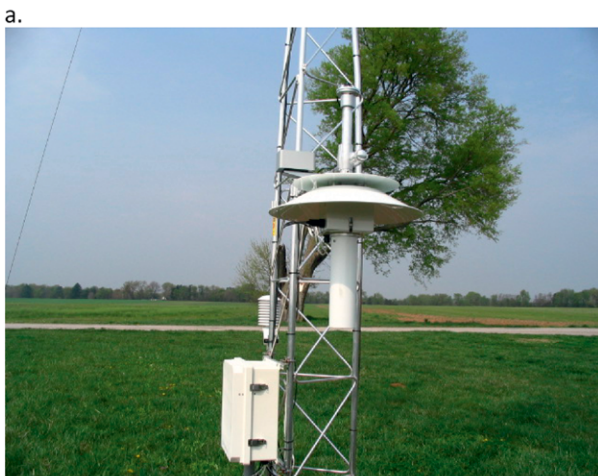
FIG. 4. (a) Aspirated radiation shield (Mahmood and Foster 2008) and (b) Gill radiation shield (naturally ventilated).
