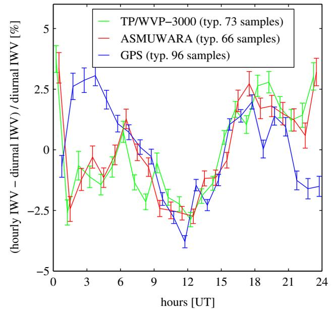
**Figure 5:** Hourly IWV means minus diurnal IWV means divided by diurnal IWV means in %, averaged over the time of the whole TUC campaign. The error bars mark the double standard error.
