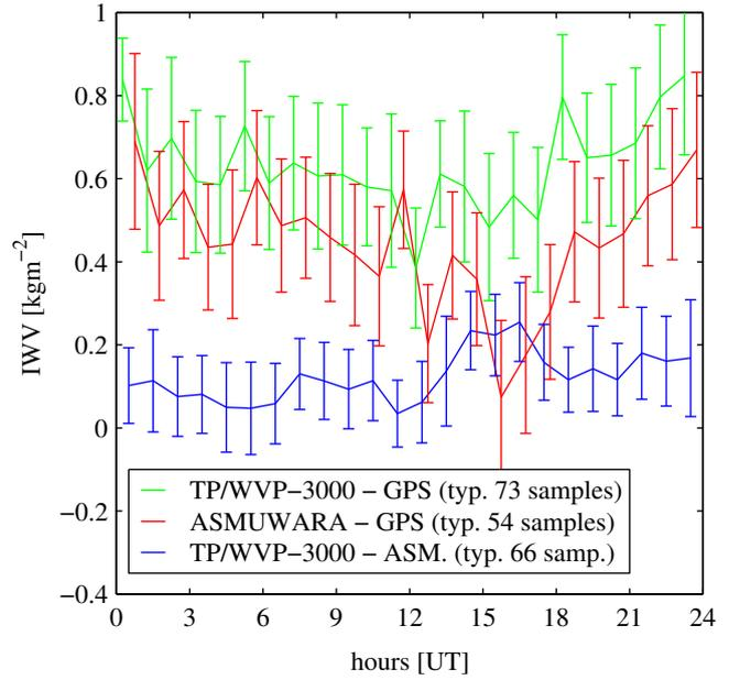
**Figure 4:** Hourly IWV differences between two instruments, averaged over the time of the whole TUC campaign. The error bars mark the double standard error.
