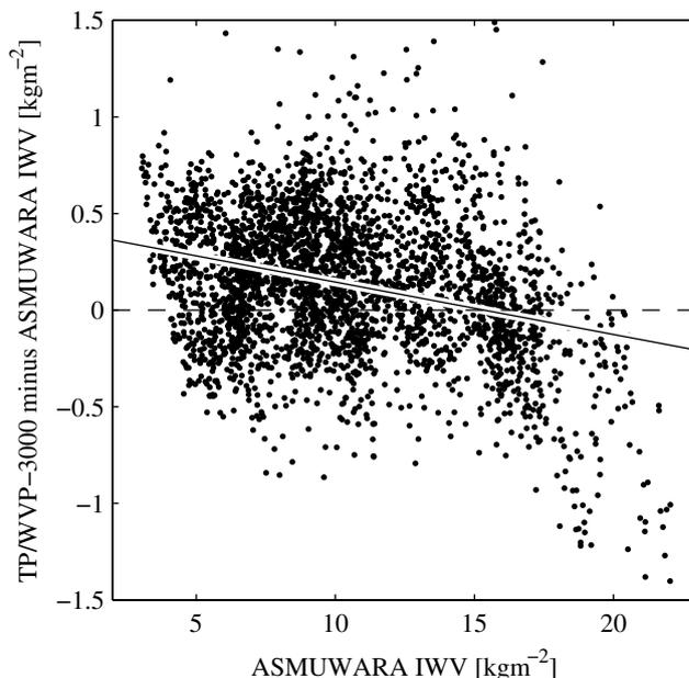
Figure 6: TP/WVP-3000 derived IWV minus ASMUWARA derived IWV. Numerical values are given in Table 3.
