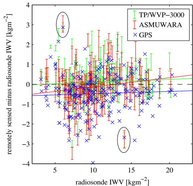
**Figure 2:** TP/WVP-3000, ASMUWARA, and GPS derived IWV minus radiosonde derived IWV. The error bars mark the double standard deviation of the radiometer data averaged over the time of the corresponding radiosonde ascent. The black ellipses mark two samples where the radiosonde has a strong bias with respect to the three other instruments. Numerical values are given in Table 1.
