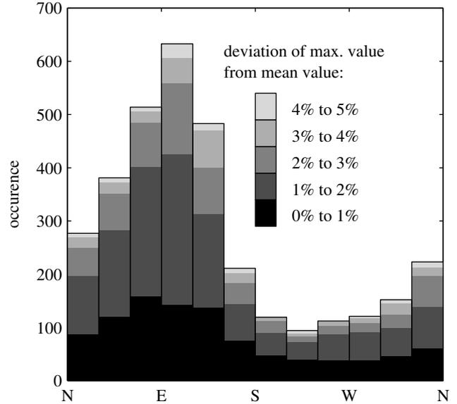
**Figure 8:** Histogram of the direction of the maximum IWV value measured with the ASMUWARA radiometer during the whole TUC campaign. The grey scale quantifies how much the maximum value exceeds the mean value.
