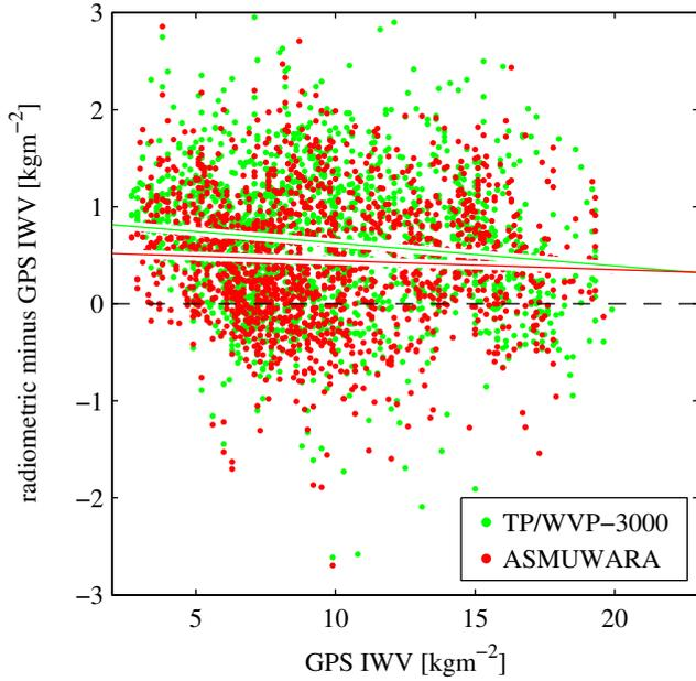
**Figure 3:** TP/WVP-3000 and ASMUWARA derived IWV minus GPS derived IWV. Numerical values are given in Table 2.
