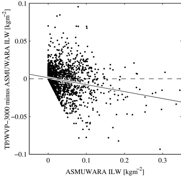
**Figure 7:** TP/WVP-3000 derived ILW minus ASMUWARA derived ILW. Numerical values are given in Table 4.
