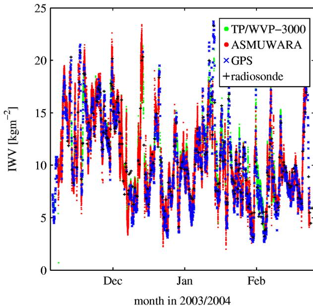
**Figure 1:** Overview of the IWV measurements made with two radiometers (TP/WVP-3000 and ASMUWARA), GPS, and radiosondes during the TUC campaign in winter 2003/2004 in Payerne, Switzerland
