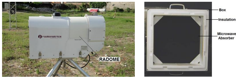
Figure 3. (a) MP3000A microwave radiometer profiler. (b) Cryogenic target for radiometer calibration.
