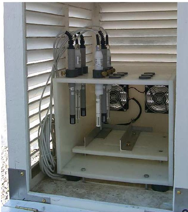
**Figure 6.** The ARM SurTHref system, showing the outer NWS-type instrument shelter and inner ventilated chamber containing six T/RH probes from two manufacturers, in which an active radiosonde is placed prior to launch for comparative measurements. A switch is activated by the radiosonde that sets a flag in the SurTHref data stream that indicates the presence of a radiosonde.
