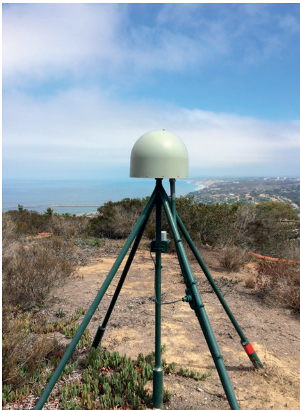
FIG. 1. A typical continuous GPS station in Southern California. [Photo credit: D. Glen Offield, Scripps Institution of Oceanography]
