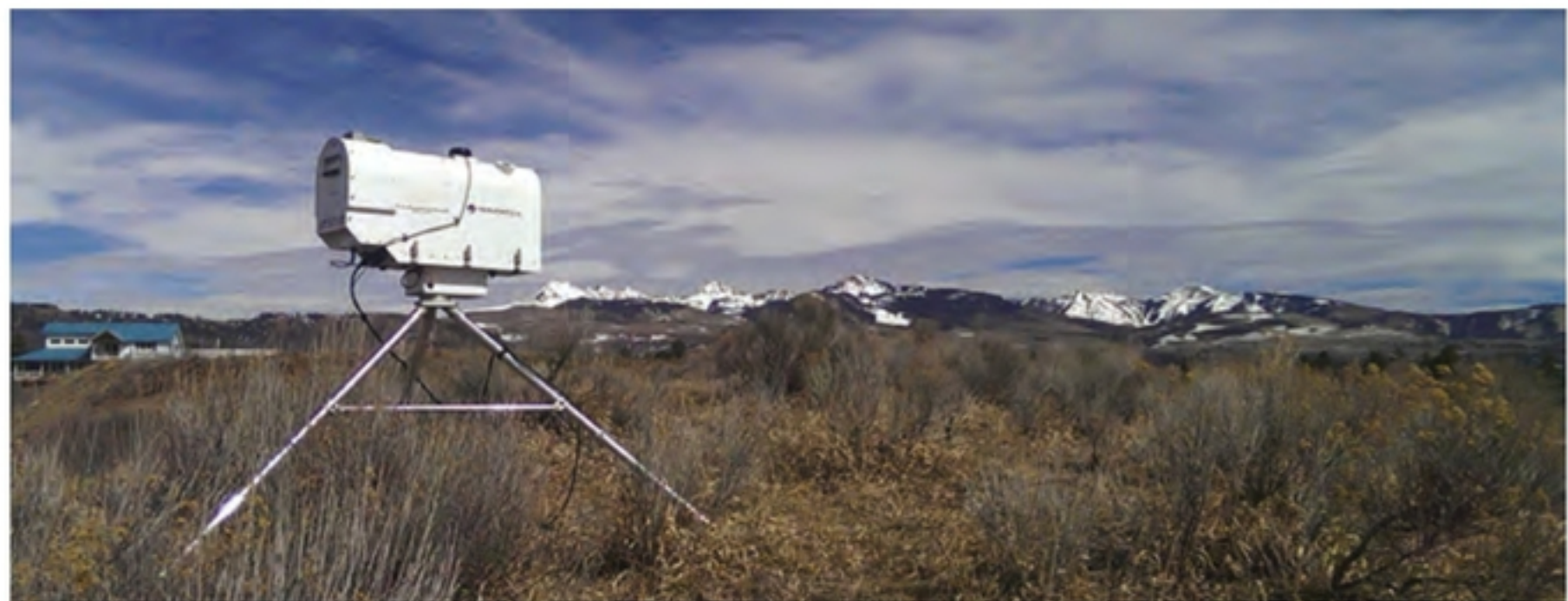
Figure 1: The Radiometrics MP-3000A microwave radiometer, installed in wintertime cloud seeding program (photo: Marta Nelson, Radiometrics staff meteorologist)
