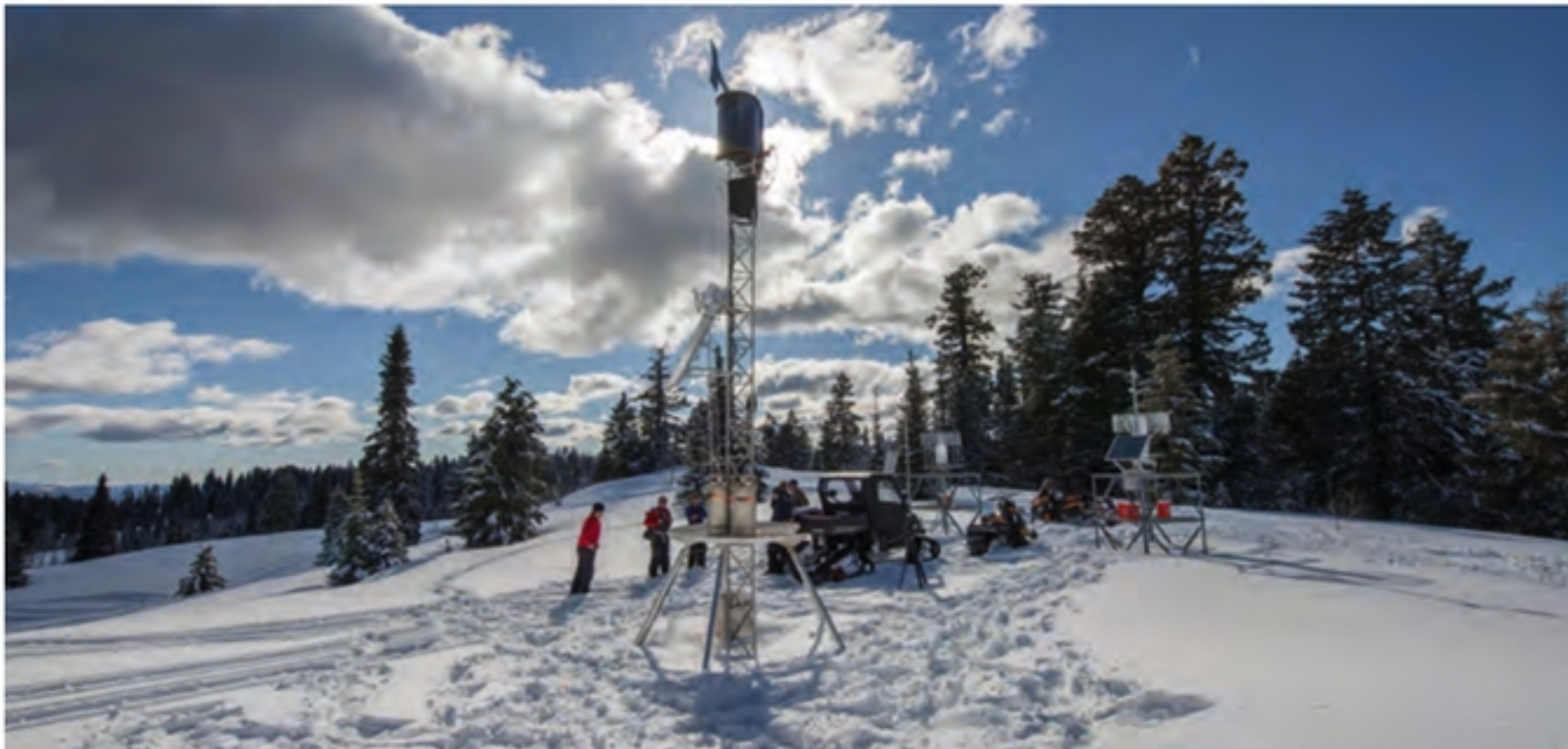
Figure 2: Ground-based seeding generator and meteorological tower (photo: Idaho Power Company)
