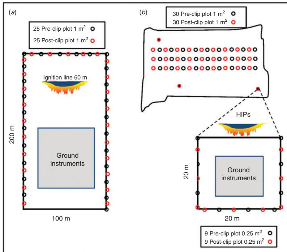
**Fig. 4.** Plot layout for (a) small replicate prescribed fires; and (b) large operational prescribed fires with sample units for the 2012 RxCADRE burns. Only large operational burns were established in the 2008 and 2011 research burns (HIP, highly instrumented plot).
