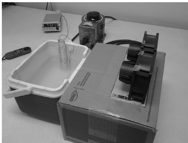
FIG. 2. Laboratory test setup. Airflow was from right to left with the fans running. Air speeds were measured at points along the long edge of the container farthest from the fans.
