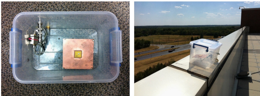
Fig. 2. The left photograph is a top-down view of the system front end. A GPS patch antenna is mounted on a 100\text{ mm}^2 ground plane and is connected via a short coaxial hardline to a low-noise amplifier and filter. The right photograph shows the antenna as it was positioned during observations. The antenna was oriented vertically, giving a maximum antenna gain in the vertical direction and a gain reduction in the horizontal direction of approximately 10 dB.
