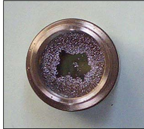
Figure 7. IRT lens showing lens pitting and extreme failure of lens coating.
