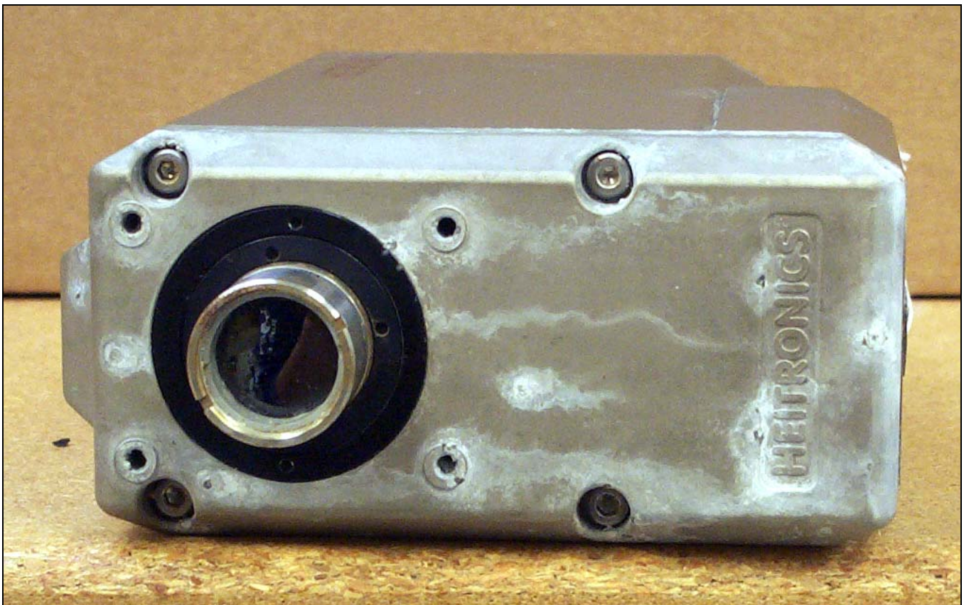
Figure 3. Typical outer housing corrosion and oxidation observed on externally mounted IRT's.
