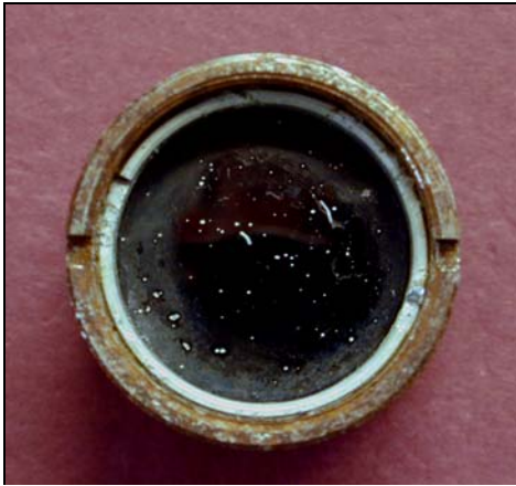
Figure 6. IRT lens showing lens pitting and lens housing corrosion.
