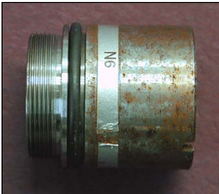
Figure 6. IRT lens showing lens pitting and lens housing corrosion.
