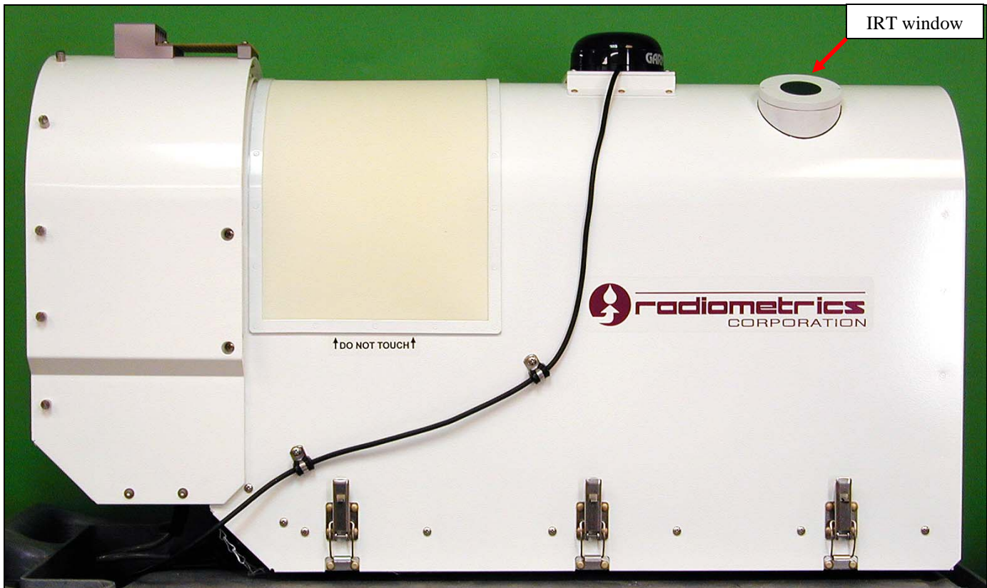
Figure 12. "A Series" radiometer cabinet hood view with IRT window.
