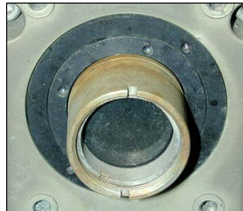
Figure 9. IRT lens showing pollutant build-up and corrosion of lens housing.
