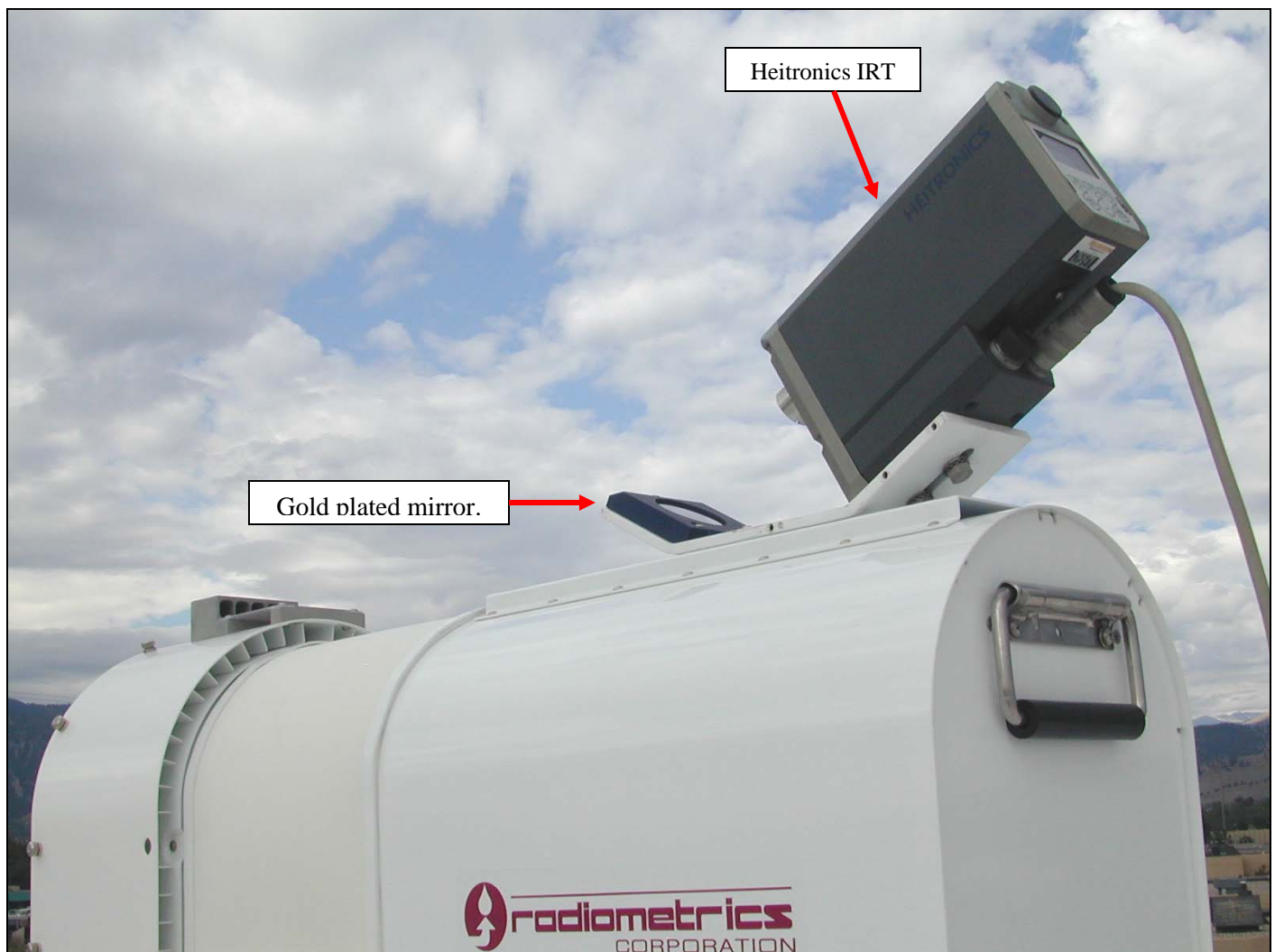
Figure 1. Older model radiometer shown with externally mounted IRT with IRT Cover removed.
