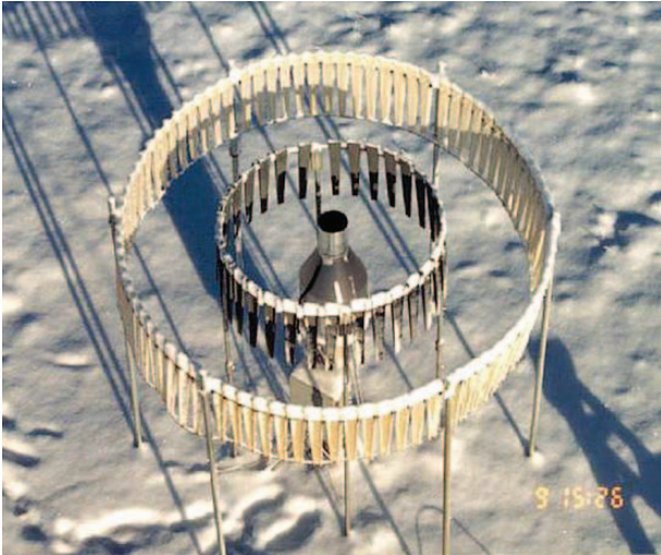
FIG. 7. Double Alter shield with GEONOR gauge in the center at the Marshall Field Site.
