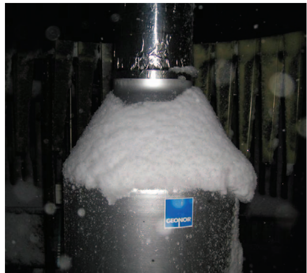
FIG. 20. Heated GEONOR inside the DFIR shield during the 17–19 Mar blizzard.
