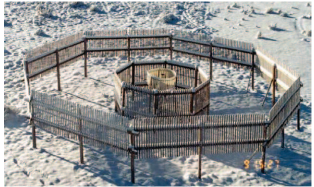
FIG. 8. DFIR shield with GEONOR in an Alter shield in the center at the Marshall Field site.
