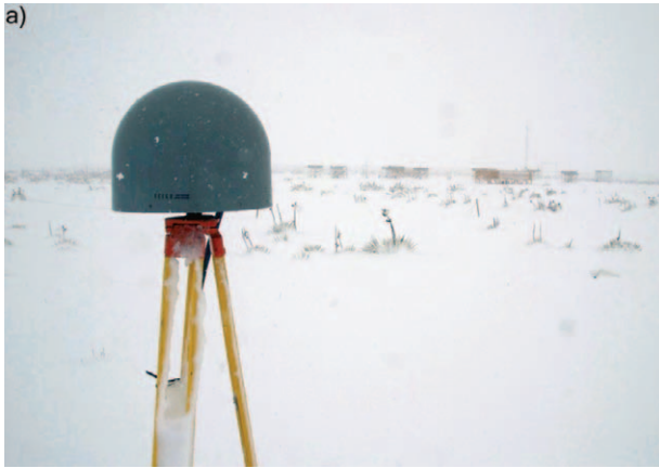
FIG. 26. (a) GPS antenna at the Marshall Field Site during a snow event. (b) Comparison of snow depth measurements over time made by manual measurements (black diamonds), automated ultrasonic instruments (grey lines), and the GPS (red dots). The variation in the GPS measurements is caused partially by real spatial variability.
