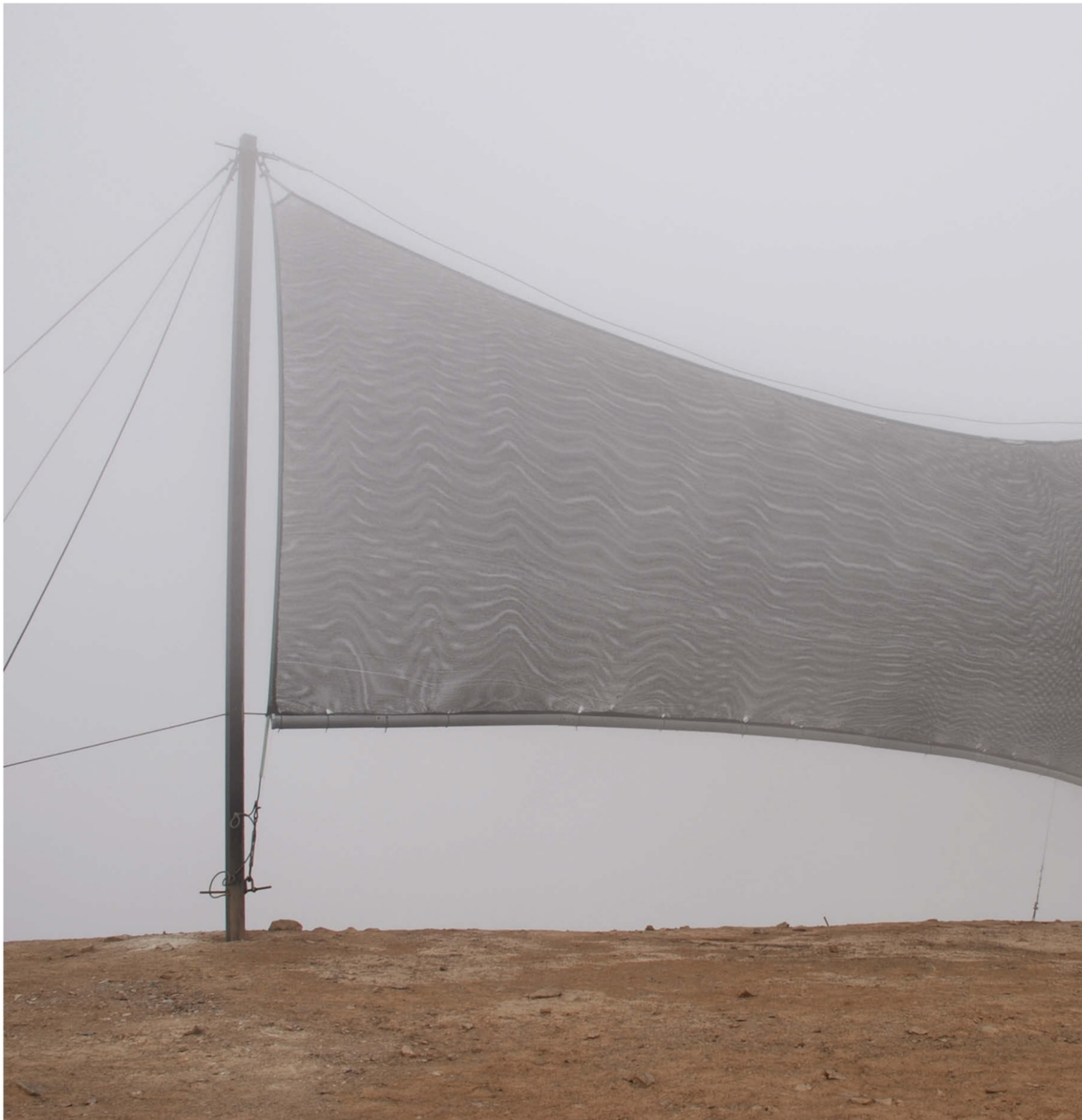
Large fog collector at the Atacama Desert Center research site in northern Chile (Photo: FogQuest/Robert Schemenauer)
