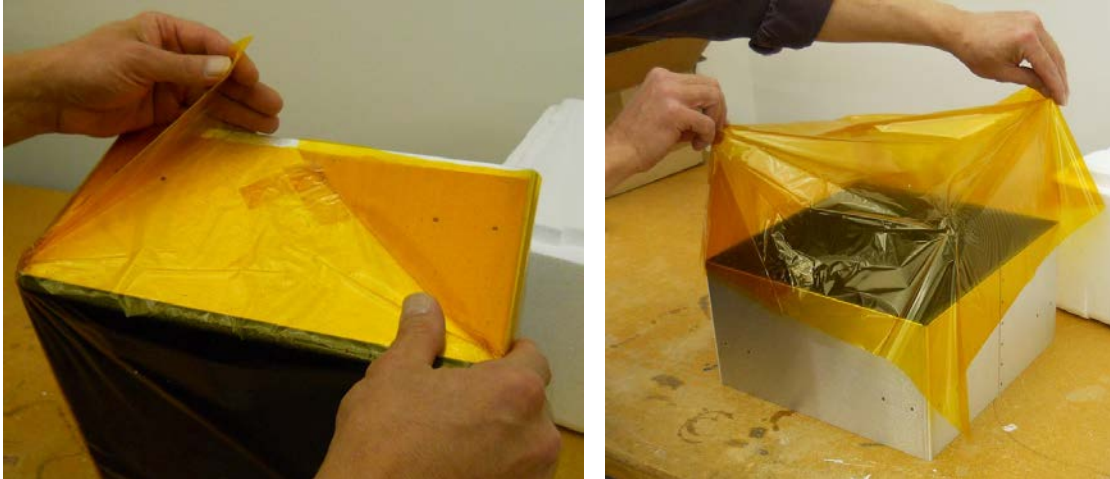
Figure 4. Untaping and removing protective liner
