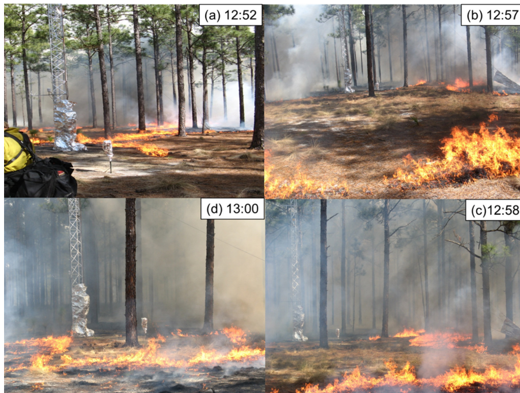
Fig. 3. Photographs showing (a) SJ10 tower, heat flux sensor box in front of the tower, and blackline ignited downwind side of the tower; (b) a line of strip head fire ignited upwind of the tower; (c) and (d) flames engulfing the tower and heat flux sensors.
