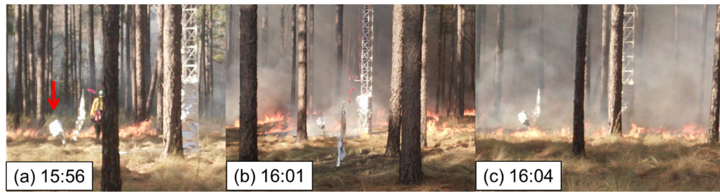
Fig. 4. Photographs showing SJ11 tower, heat flux sensor box (indicated with a red arrow), blackline ignited around the tower, and backing fire approaching to the tower. (For interpretation of the references to color in this figure legend, the reader is referred to the web version of this article.)
