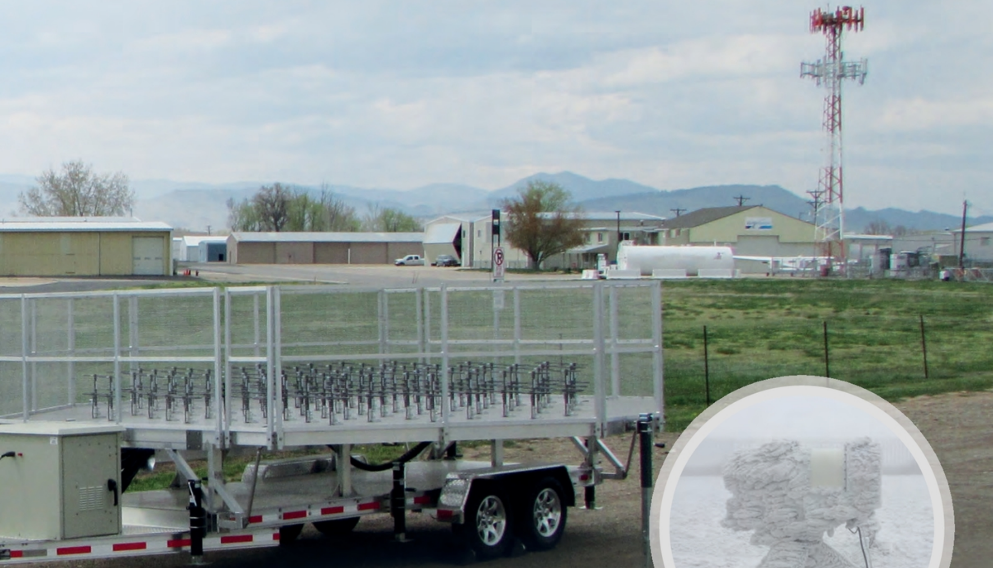
↑ Figure 1: Mobile SkyCast system at a regional airport: Raptor XBS-T with phased array antenna, MP-3000A MWR, and central processing shelter
