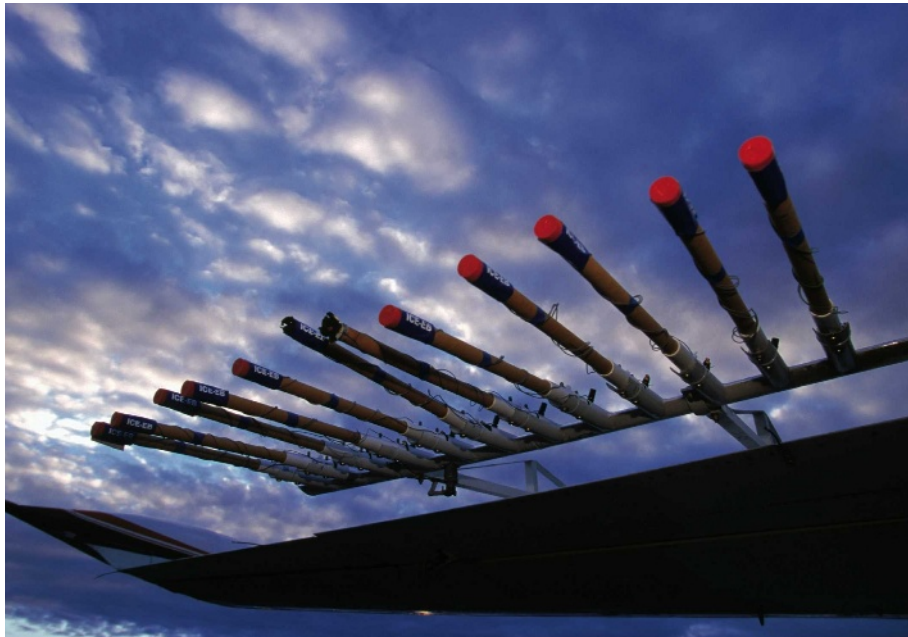
Light aircraft are used to seed clouds with compounds such as silver iodide.
