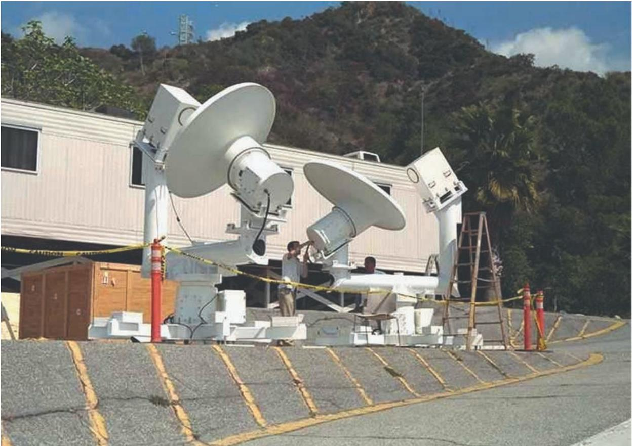
**Figure 1.** Two AWVRs during assembly at JPL.
