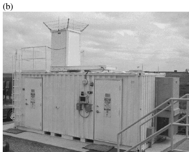
FIG. 1. Pictures of (a) the AERI and (b) Raman lidar at the ARM Southern Great Plains Cloud and Radiation Testbed site. The AERI system is 1 m × 1 m × 0.5 m in volume and weighs approximately 250 lb. The Raman lidar is housed in a 6.1 m × 2.4 m × 2.4 m seatainer.
