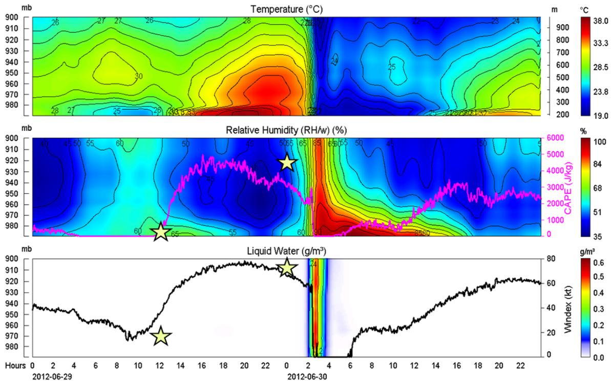
**Figure 1. Radiometer profiles to 1 km height with superimposed CAPE and Windex derived from radiometer and radiosonde (stars) data<sup>4</sup>.**
