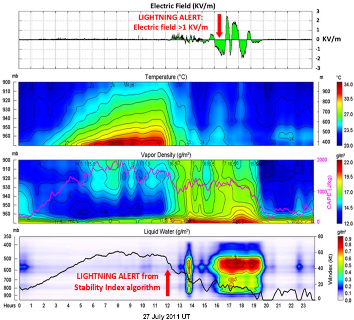
Figure 2. Lightning alerts from electric field and thermodynamic measurements.<sup>5</sup>
