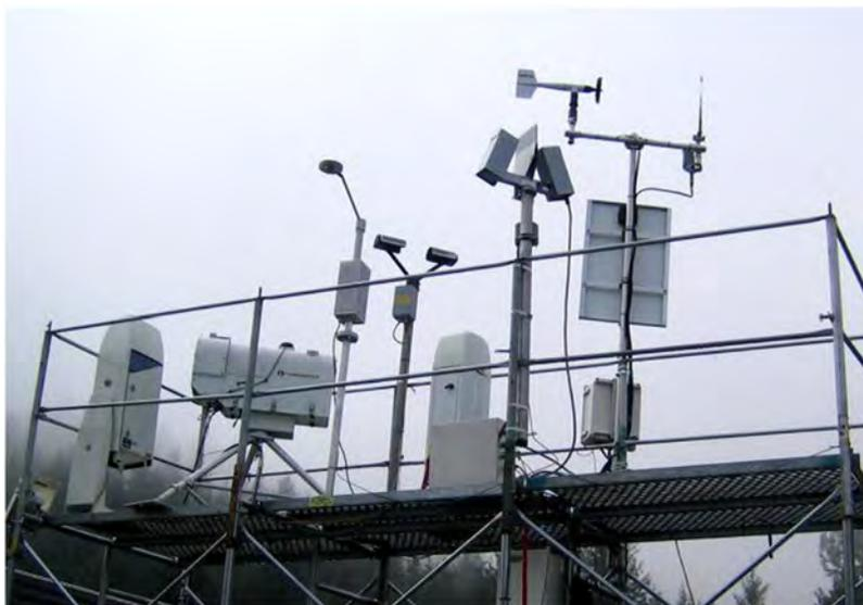
Fig. 2. Microwave profiler (second from left) and other meteorological sensors.
