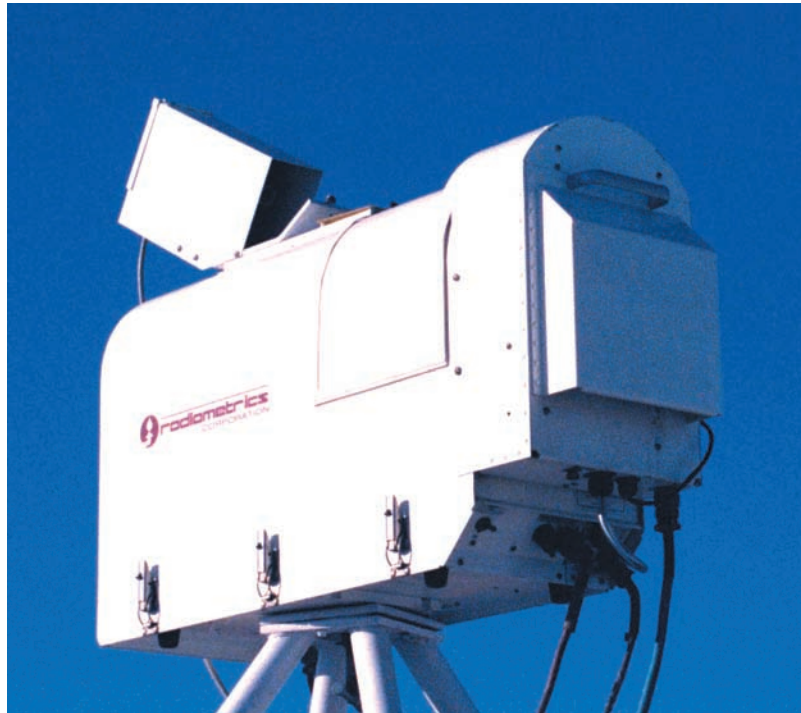
Figure 1. Radiometric profiler (Radiometrics TP/WVP-3000) with 12 microwave and 1 infrared observation channels.
