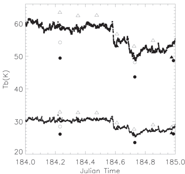
Figure 17. The 24-hr time series of T_b at 23.8 GHz (*) and 31.4 GHz (+) on July 3, 1999. The closed circles were calculated from the original ARCS-2 radiosondes (age = 315 days). The open circles were calculated from corrected ARCS-2 radiosondes. The closed triangles were calculated from the original RHB radiosondes (age = 172 days). The open triangles were calculated from corrected RHB radiosondes. The RTE model [5] was used (after [28]).
