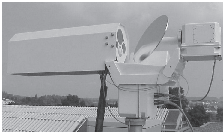
Figure 3. The ASMUWARA in operation in Bern. The openings of the four horns appear as grey disks at the left of the rotatable mirror, while the IR radiometer looks through the white cylinder below the largest horn.
