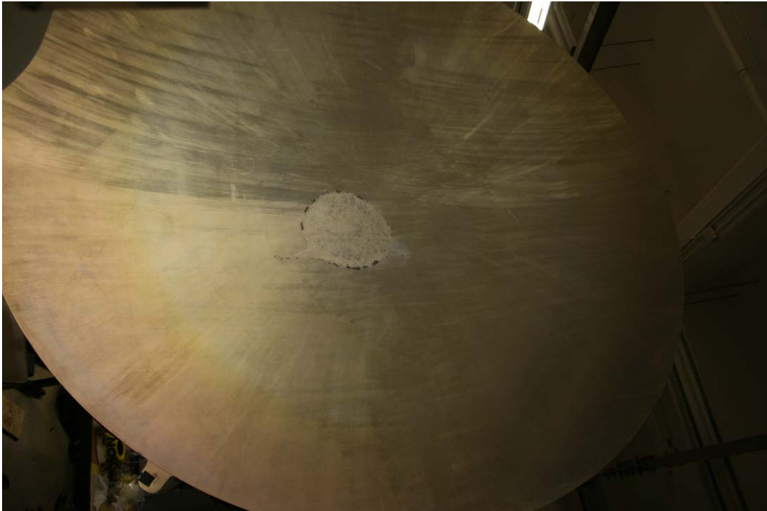
Figure 2.4: Large discoloration in the middle of the primary mirror is oxidation of the Aluminum layer from water that was allowed to pool during long term storage. This blemish caused an \sim 5 K polarized offset.
