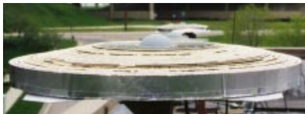
Figure 1. Ground reflected multipath was minimized using choke ring antennas augmented with ring shaped collars 25 cm in width.
