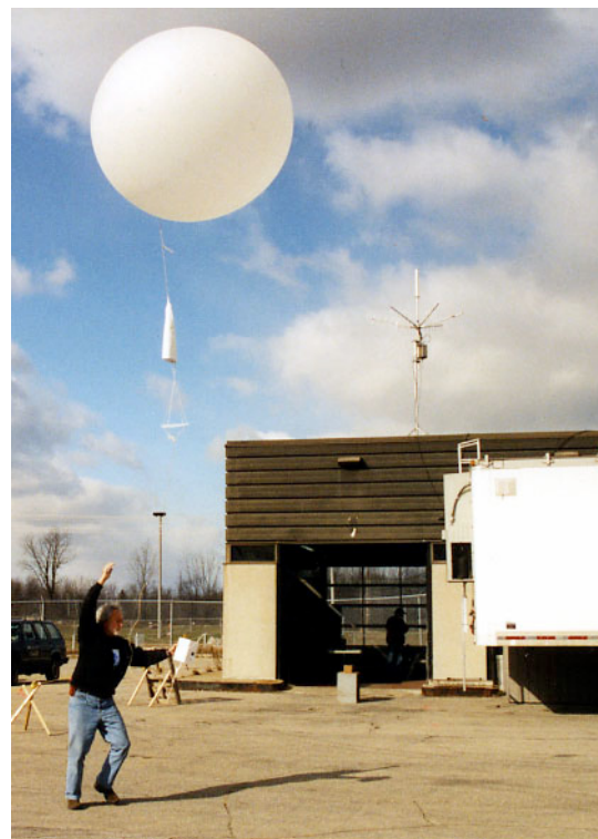
Figure 2, Launch of balloonsonde at Mirabel Airport, multi-element direction antenna is visible on the building roof.
