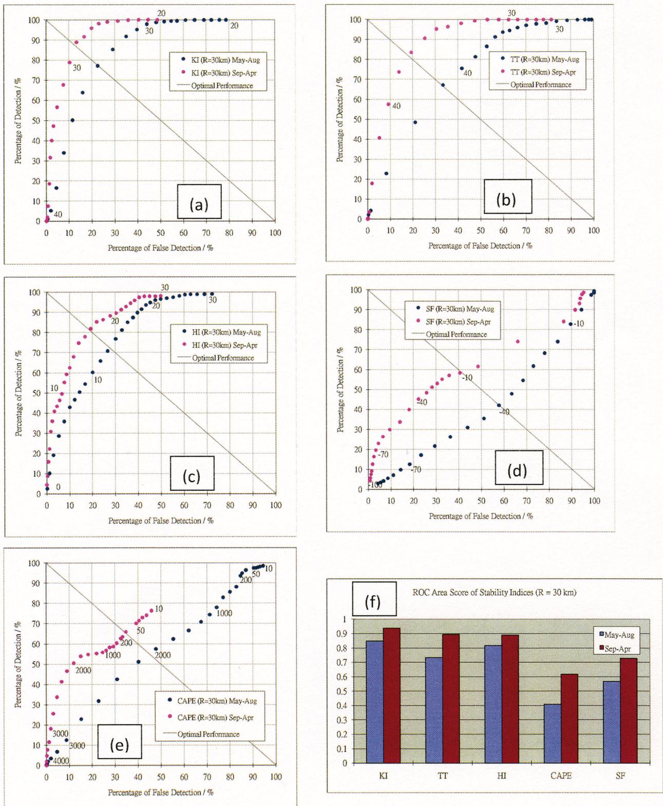
**Figure 4:** (a) to (e) are the ROC curves for various radiometer-based instability indices for summer (May to August) and non-summer (September to April) periods, including K index, TT, HI, SF and CAPE. (f) gives the areas under the ROC curves.
