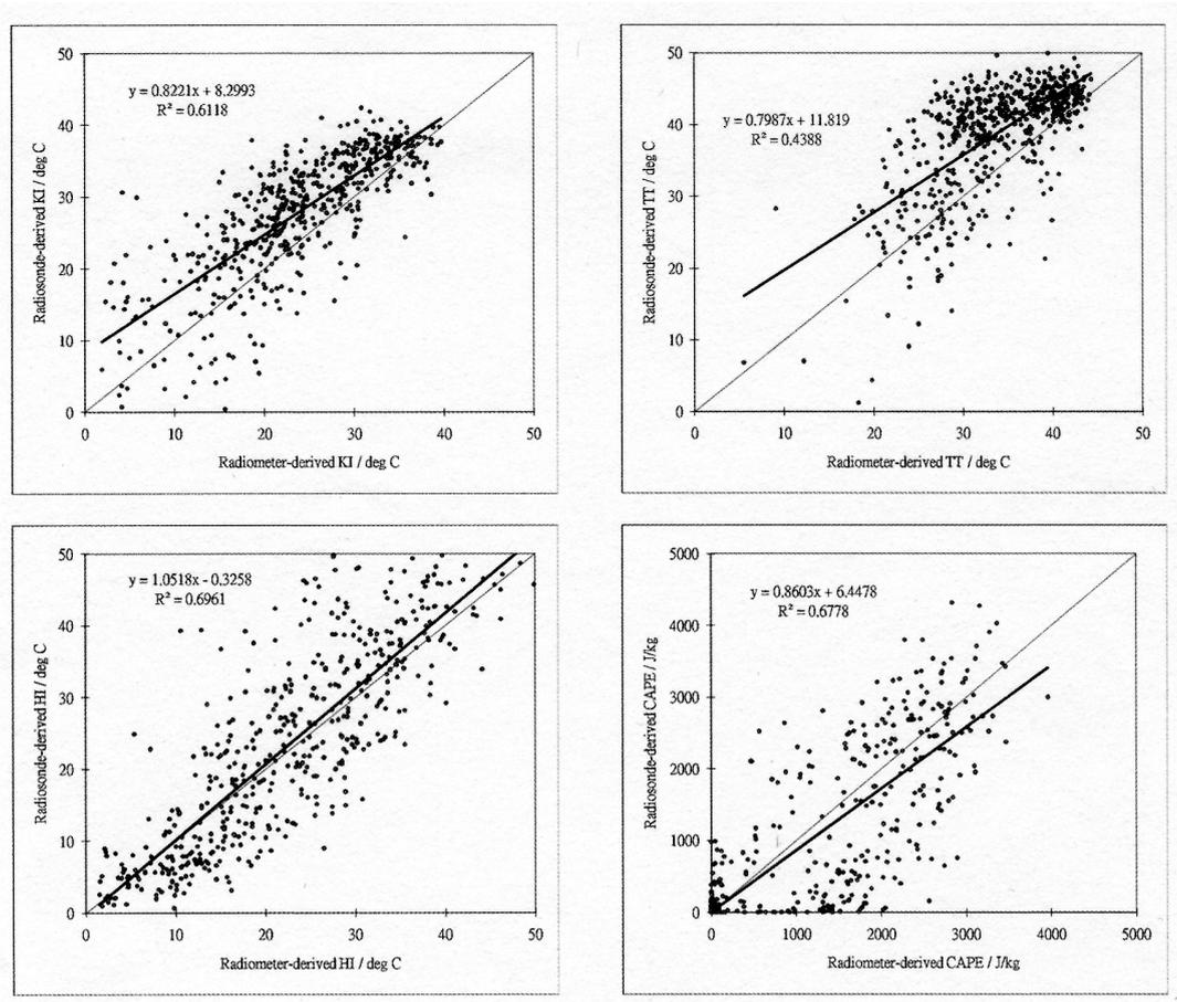
**Figure 2:** Comparison of the instability indices derived from the radiometer and radiosonde: K index, TT, HI and CAPE.
