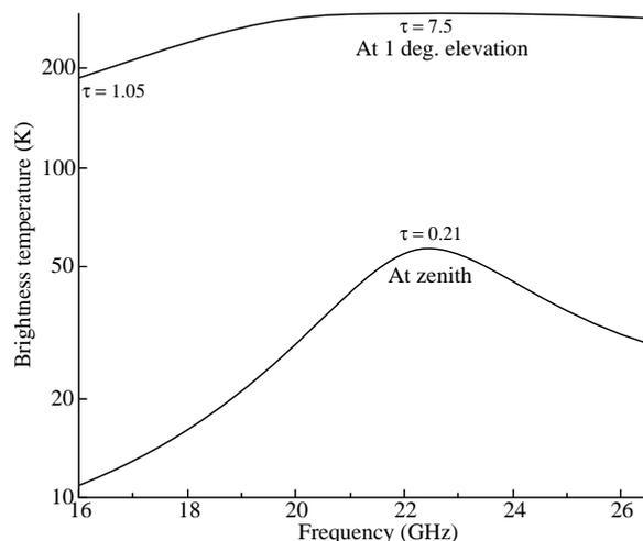
Fig. 1: Brightness temperature as a function of frequency for a cloud-free atmosphere typical of summer conditions ( $22^\circ\text{C}$  surface temperature and  $30\text{ kg/m}^2$  of precipitable water) for a ground-based radiometer pointing at zenith (lower curve) and  $1^\circ$  elevation (upper curve). The optical paths  $\tau$  at the frequencies of minimum and maximum attenuation are also indicated.
