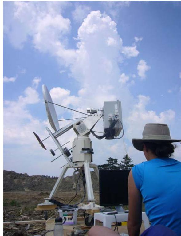
Fig. 3: The prototype of the mesoscale radiometer.
