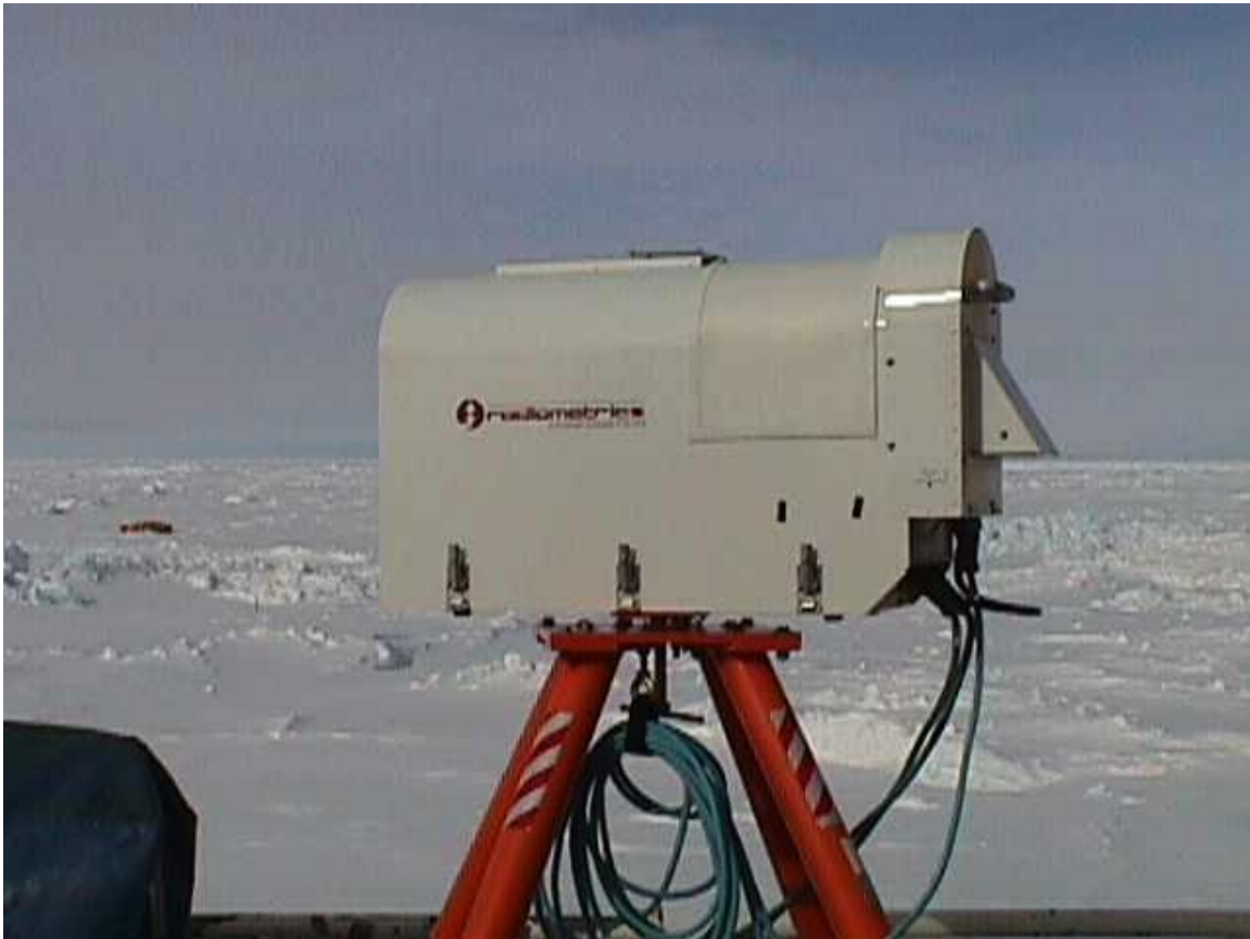
Figure 1. The ARM microwave radiometer deployed at SHEBA.
