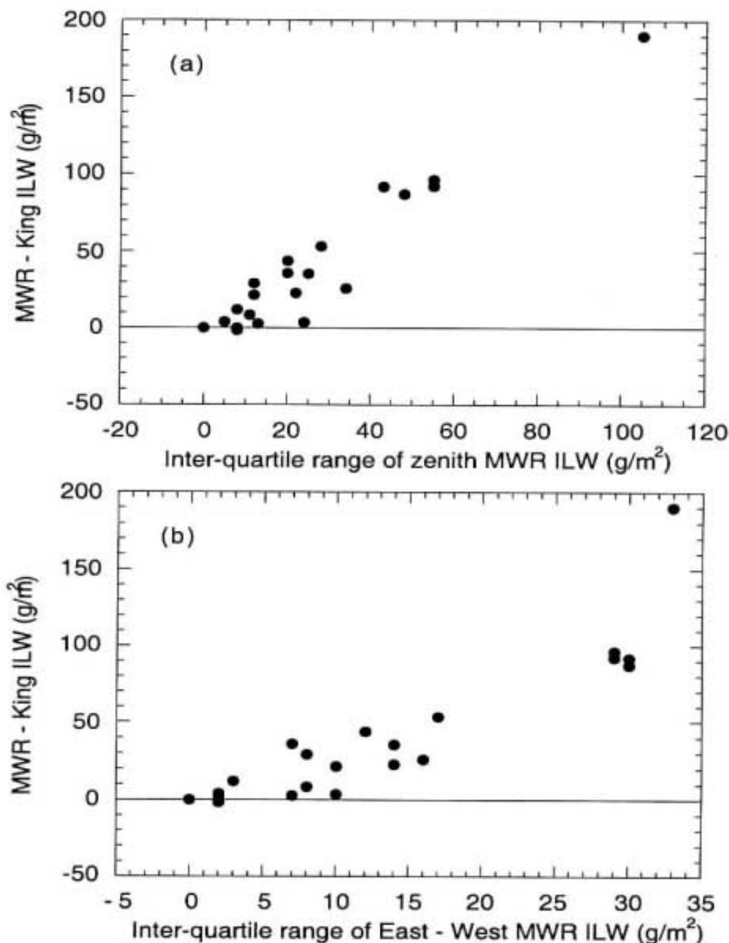
**Figure 6.** Differences in integrated liquid water (ILW) from the microwave radiometer (MWR) and the King probe on the NCAR C-130 plotted against (a) the temporal variation in ILW from the MWR described by the inter-quartile range (75<sup>th</sup> percentile – 25% percentile) of ILW; (b) the spatial variation in ILW described by the inter-quartile range of the difference in ILW measured at 45° angles on either side of zenith.
