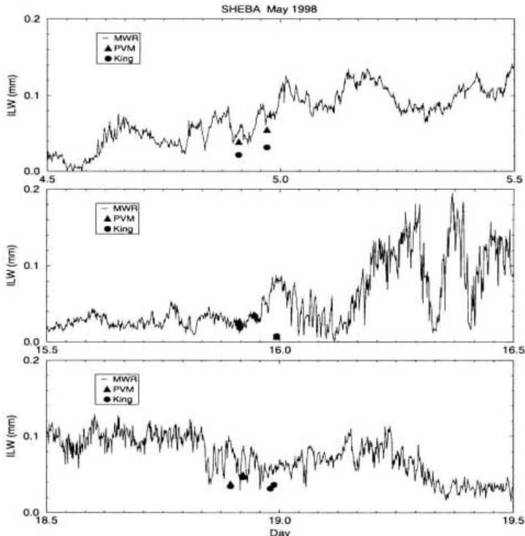
**Figure 4.** Time series of integrated liquid water (ILW) from the microwave radiometer for days when the NCAR C-130 aircraft with the PVM and King liquid water probes flew over the site.
