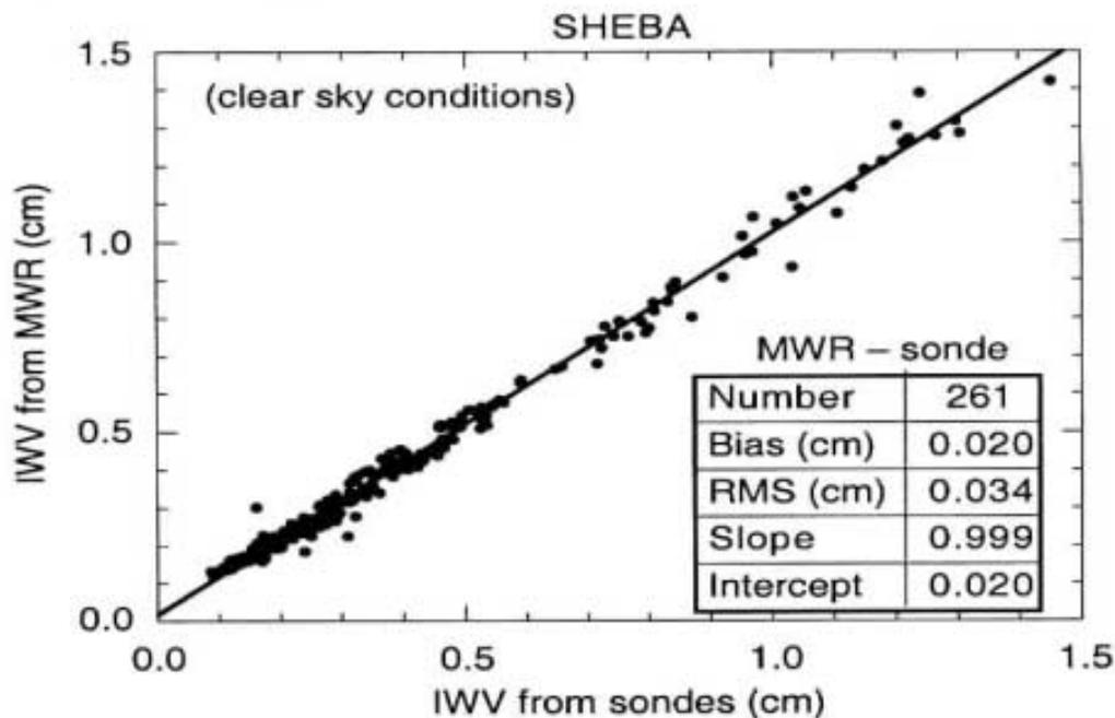
**Figure 2.** Integrated water vapor (IWV) from Vaisala radiosondes compared with 30-minute averaged values from the microwave radiometer (MWR) during clear sky conditions for December 1997 - September 1998.
