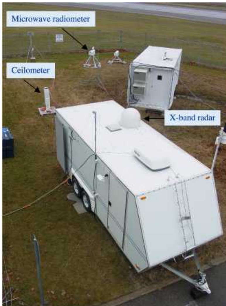
Figure 1.—NASA Icing Remote Sensing hardware as installed for the AIRS II field test program.
