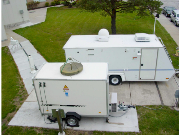
Figure 3.—NASA's icing remote sensing site. Includes the larger trailer which houses the X-band radar (under the radome) and the instrument computers, the Radiometrics 3000 series radiometer at the top left, the Vaisala ceilometer to the left, and the Metek Ka-band radar housed in the smaller trailer at the bottom of the photo.
