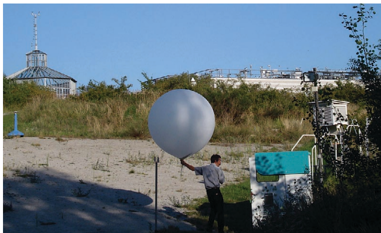
FIG. 2. The Deutscher Wetterdienst’s Meteorologisches Observatorium Lindenberg, designated as GRUAN Lead Center and the first GRUAN network station, has all the GRUAN observational capabilities depicted in Fig. 1. Here Michael Schröter prepares to launch a radiosonde and verifies that the ground station is receiving data from the sonde. A Stevenson shelter (behind bushes at lower right) houses reference surface instruments for comparison. On the roof of the radiation building (in background on right) are Baseline Surface Radiation Network instruments (pyranometer, pyrliometer, pyrgometer, and all-sky camera) and a microwave radiometer (far right). A GSNN antenna is to the left of the radiation building. The historic winch house (in background on left) was used in the nineteenth and twentieth centuries for meteorological profile observations with tethered aerological kites; the observatory holds the world record for achieving a kite altitude of 9,750 m on 1 Aug 1919.
