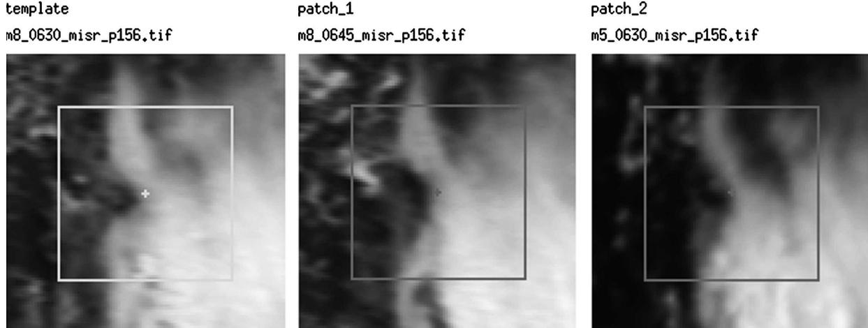
FIG. 6. MPGC triplet matching between (left) *Meteosat-8* HRV at time  $t$ , (middle) *Meteosat-8* HRV at time  $t + 15$  min, and (right) *Meteosat-5*. The template and patch windows are shown as gray squares. It can be seen that there are larger differences in the cloud structures between *Meteosat-8* HRV at time (left)  $t$  and at (middle)  $t + 15$  min, resulting from changes within the 15-min time interval.
