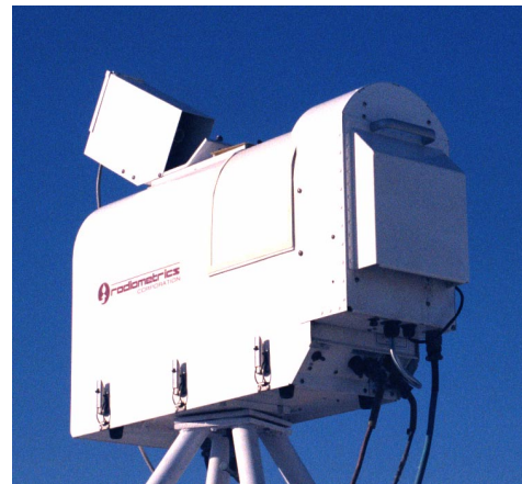
Figure 1. Radiometric profiler < http://radiometrics.com >.
