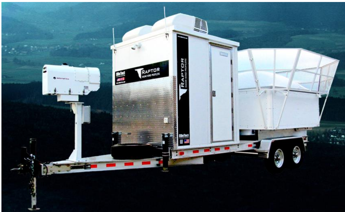
Figure 5. Mobile Radar Wind and Thermodynamic Profiler (RWTP) 16 .
