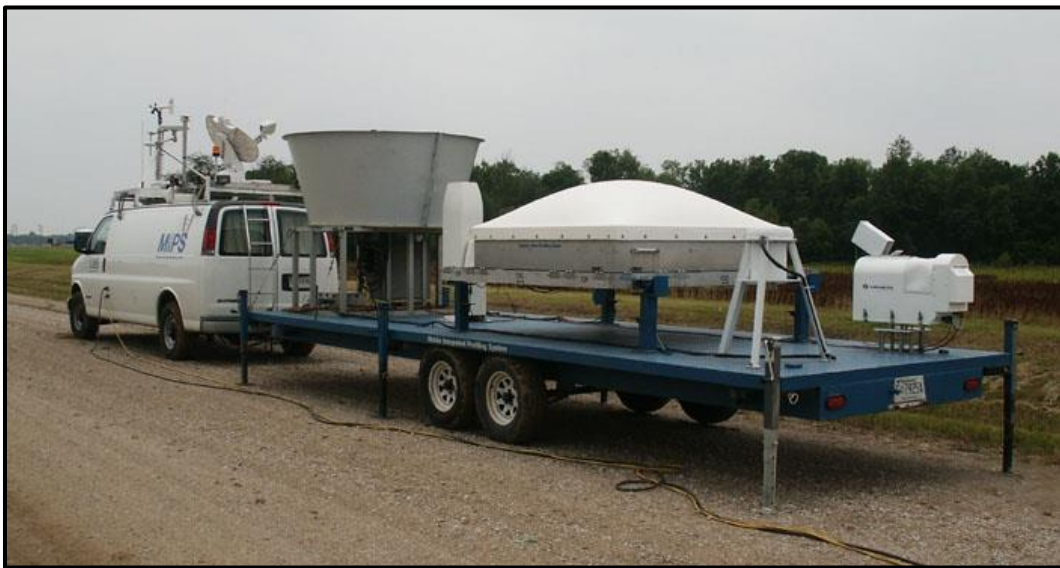
Figure 6. MIPS includes sodar, wind radar and thermodynamic profilers.
