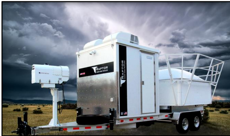
Figure 1. One of two mobile Fireweather profilers deployed by SDG&E. 1
