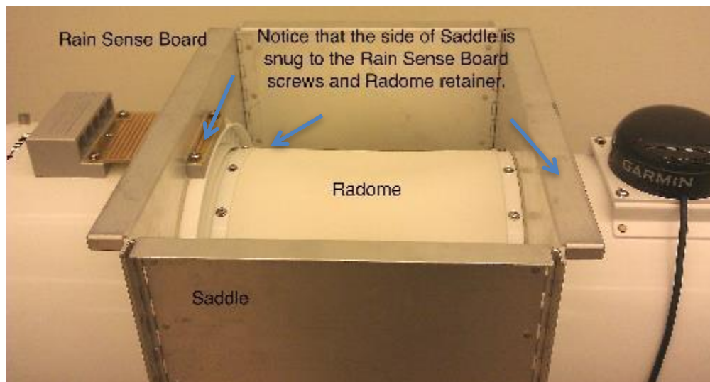
Figure C-3. Saddle for Cryogenic Target, properly seated
