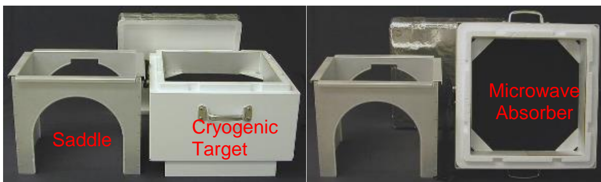
Figure C-1. Cryogenic Target for calibrating microwave-profiling radiometers
