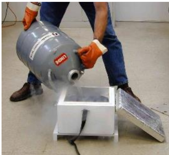
Figure C-4. Proper method for safely pouring LN2 into the Cryogenic Target
